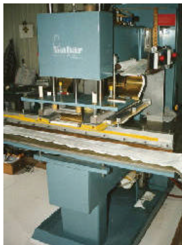
10 kW RF sealer with long sealing electrode for tent manufacturing.
