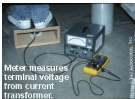
Measuring induced body current in an RF sealer operator.
