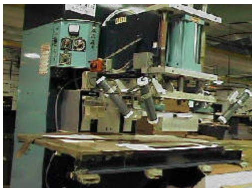
A sealer fitted with a short electrode, spotting lights. The timer controls the seal time.
