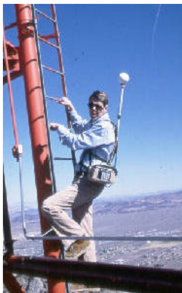
Using a back-mounted RF field probe to measure exposure while climbing.
