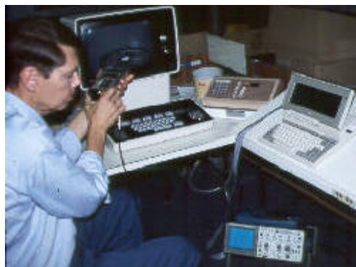
A digital oscilloscope is used to capture the waveform of the magnetic field for subsequent analysis using FFT techniques.
