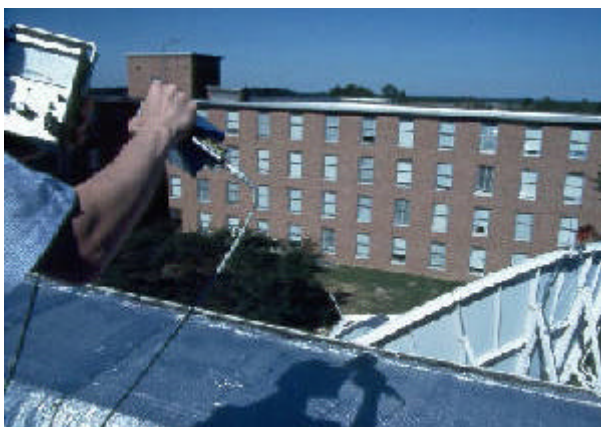
Conducting a survey of microwave field levels atop a roof at a government facility that uses an earth station for data transmission to remote locations.
