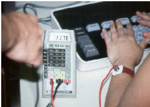
Measuring electric field induced currents in the VDT operator.
