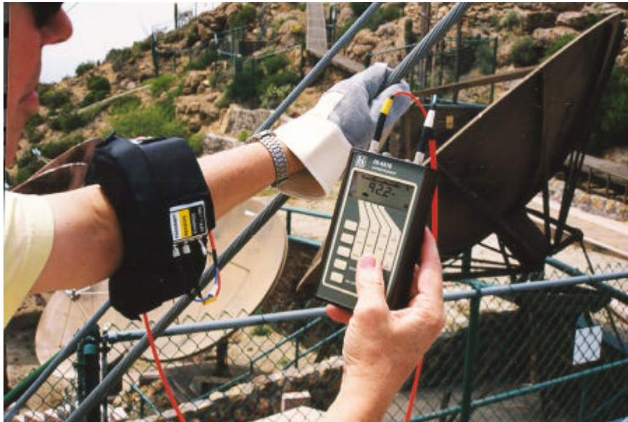
Figure 6. Grasping a guy wire with a conventional work glove and measuring the contact current flowing in the arm with the Holaday Industries clamp-on current probe.
