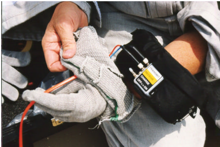
Figure 7. The conductive glove was brought up and over the current probe to allow the probe to measure the contact current flowing in the wrist and arm.
