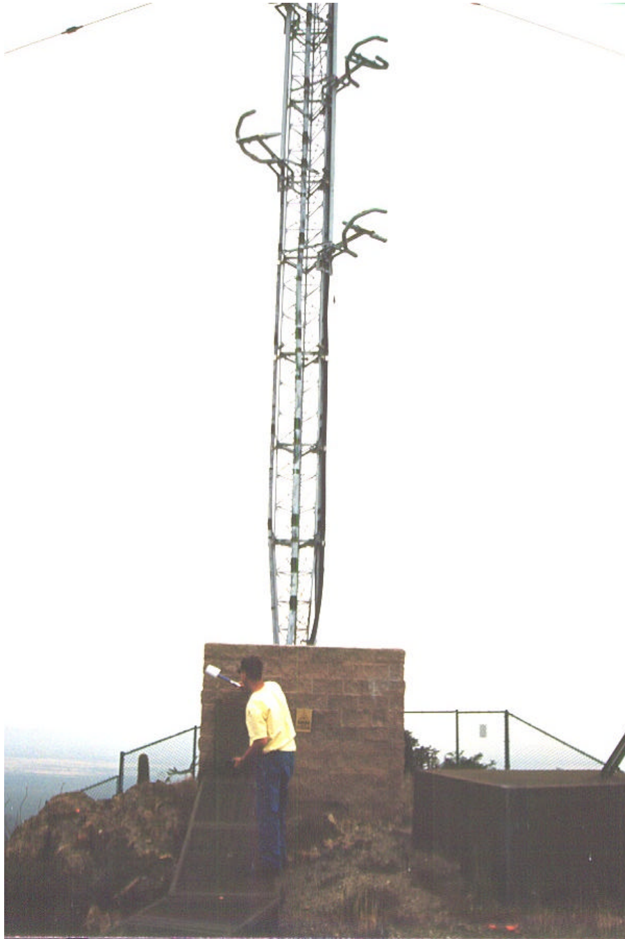
Figure 1. Induced body current measurements were performed near a tower supporting four high-power FM radio stations. Lowest element of the four antennas was 25.6 feet above ground.
