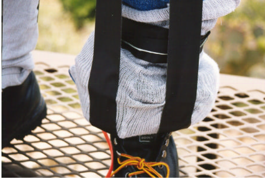
Figure 4. Nonconductive tape was used to help support the current probe just above the ankle. The fiber optic leads were routed through a small hole in the conductive sock.
