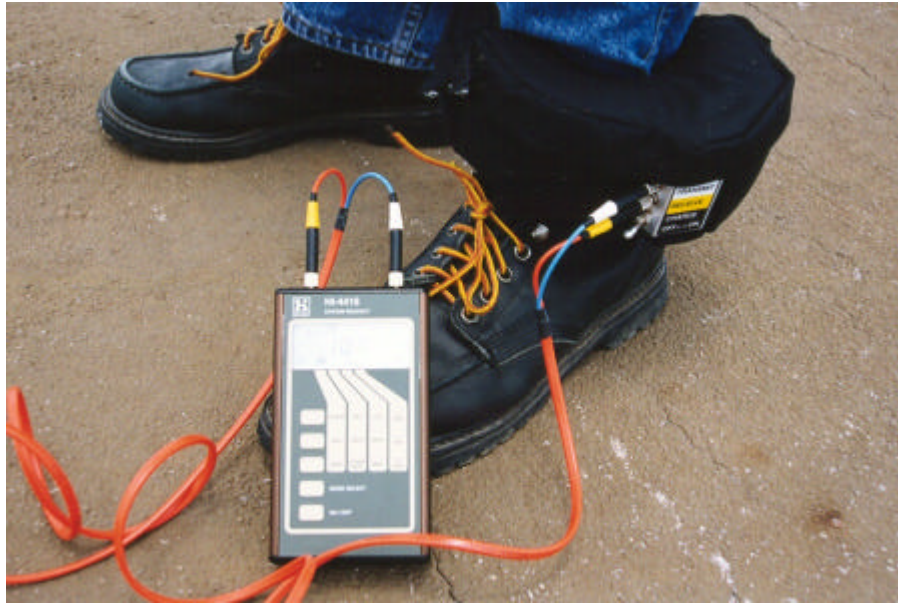
Figure 2. Holaday Industries Model HI-3702 clamp-on current probe was placed around the ankle region to measure induced body current. The remote readout module is fiber optically coupled to the current probe to avoid RF interference and distortion in current measurements.
