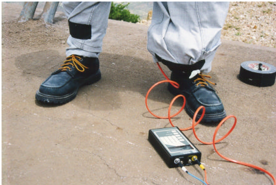
Figure 5. After attaching the current probe around the ankle and bringing the conductive sock up and over the probe, the KW-GARD™ pant leg was then brought down over the sock and probe and taped to the conductive sock just above the top of the shoe to form an electrical bond between the suit and the sock.
