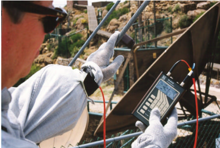
Figure 8. The sleeve of the KW-GARD™ suit was brought down and over the glove region and taped to form an electrical bond between the sleeve and glove.
