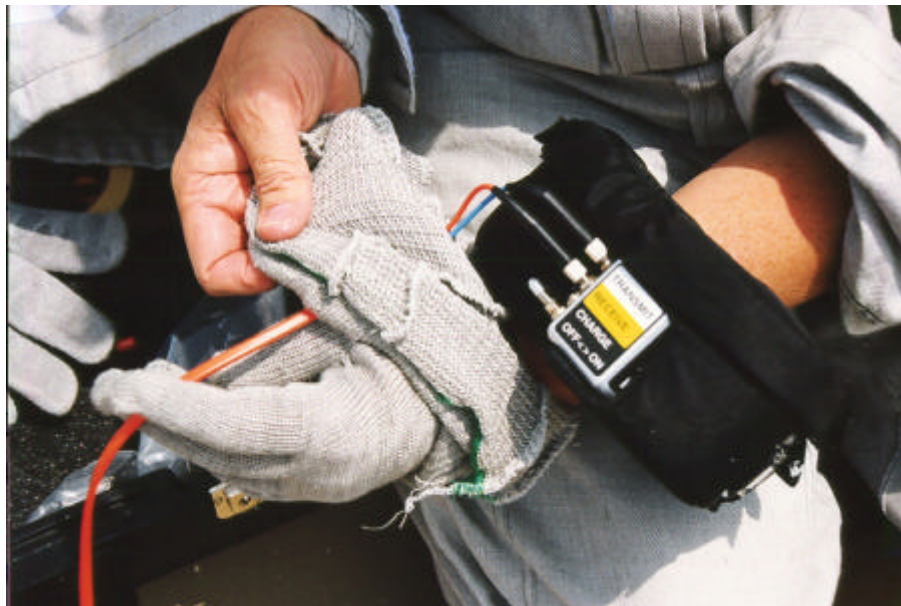
Figure 7. The enlarged conductive glove was brought up and over the current probe and then cinched tightly to the fore arm prior to bringing the sleeve down and over the glove.
