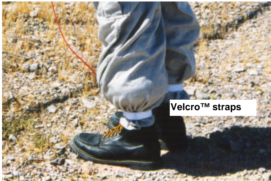
Figure 5. After attaching the current probe around the ankle and bringing the conductive sock up and over the probe, the KW-GARD™ pant leg was then brought down over the sock and probe and strapped to the conductive sock just above the top of the shoe using Velcro™ straps to form an electrical bond between the suit and the sock.
