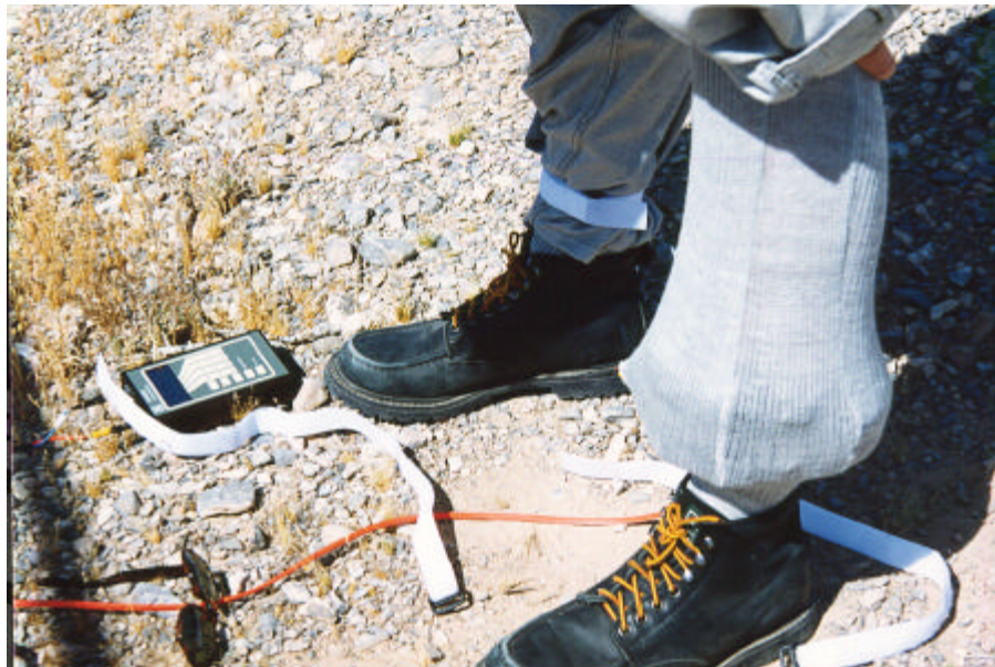
Figure 4. Velcro™ straps were used to bind the upper portion of the special sock to the calf to help support the current probe just above the ankle. The fiber optic leads were routed through a small hole in the conductive sock.
