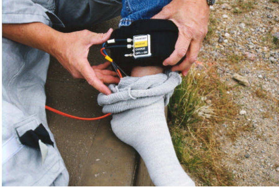
Figure 3. The current probe was placed around the ankle but beneath the conductive sock to measure the body current flowing in the ankle as opposed to the current flowing in the suit fabric.
