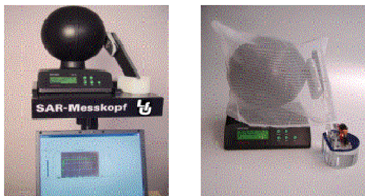
Figure 1. Left: Standard measurement kit including a SAR- measurement head, an attached computer notebook with software. Right: Example of an experimental set up.
